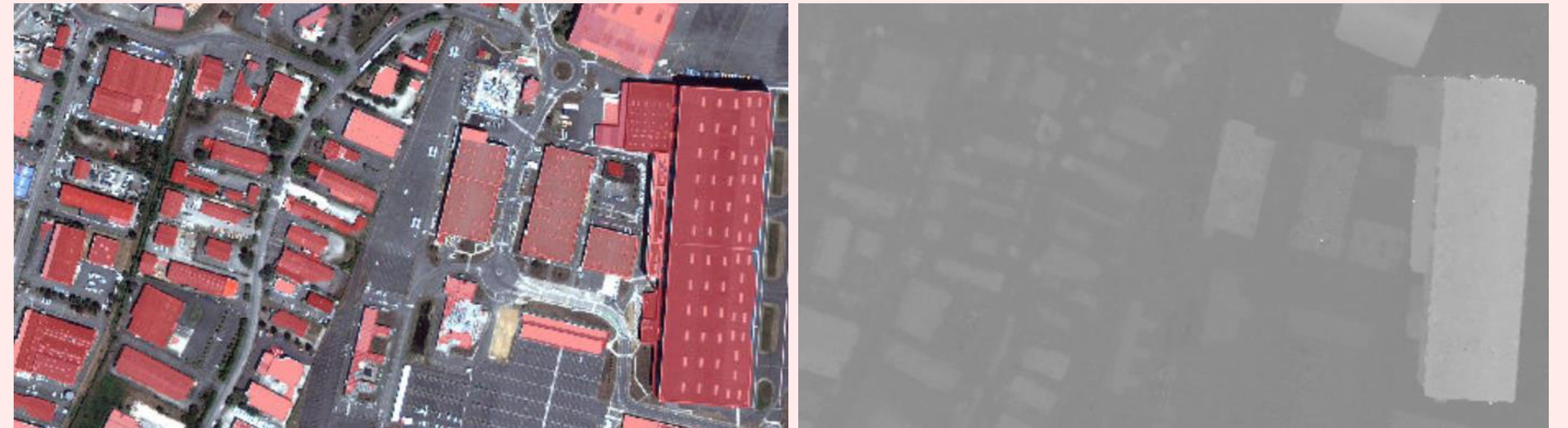
Left: Step 3 - Building Classification Map ; Right: Step 4: Digital Surface Model
